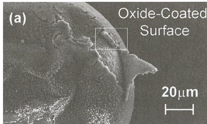
Figure 1.4: Scanning electron micrograph of a quenched 210 \mu\text{m} aluminum particle (Bucher, Ernst & Dryer 2000).
